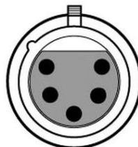
DmX Output 5 Pin XLR Socket
